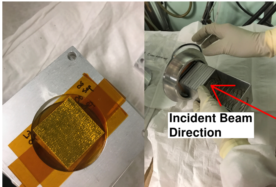
Figure 2.1: Photo of an individual foil packet secured to the aluminum sample holder (left) and the entire foil stack (right). The front of the stack (facing the beam) is oriented towards the right in this photo.
