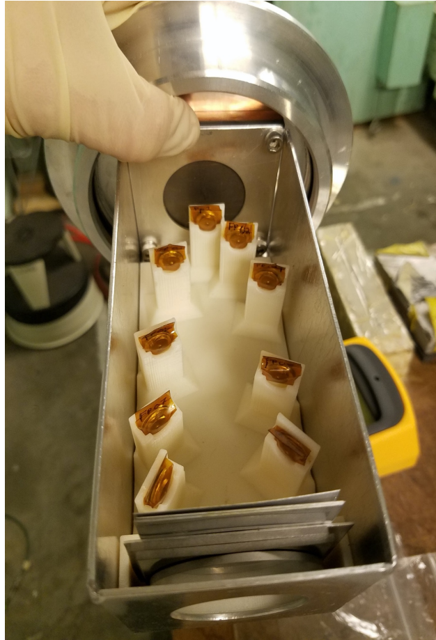
Figure 3.11: Photo of the foil holder used in the activation experiments. The plastic holder was loaded directly inside of the beam-pipe. Foils were wrapped in Kapton polyimide tape for encapsulation during handling. Thin aluminum foils were placed just behind the breakup target to prevent secondary protons from activating the samples.
