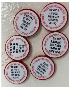
Figure C.1: Calibration sources used in the HPGe efficiency calibration work. The ^{288}\text{Th} source was not used in the analysis, as the relevant lines were obscured by background and lead scattering gammas in the measurement.
