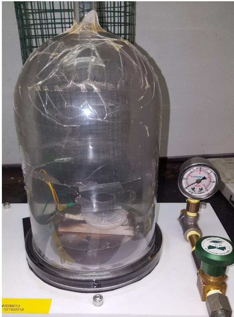
Figure 4.2: Overview of vapor deposition system contained within a bell jar cover. The glass vial and microscope slide over top the coil heater is visible within the jar.
