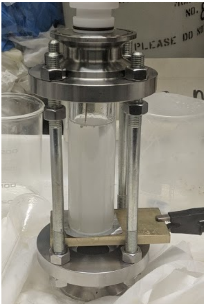
Figure 4.4: Two electrode plating cell, using a titanium backing placed on a brass cathode and under a Teflon washer and the glass vial. The platinum anode is visible at the top of the vial, touching the surface of the plating solution.
