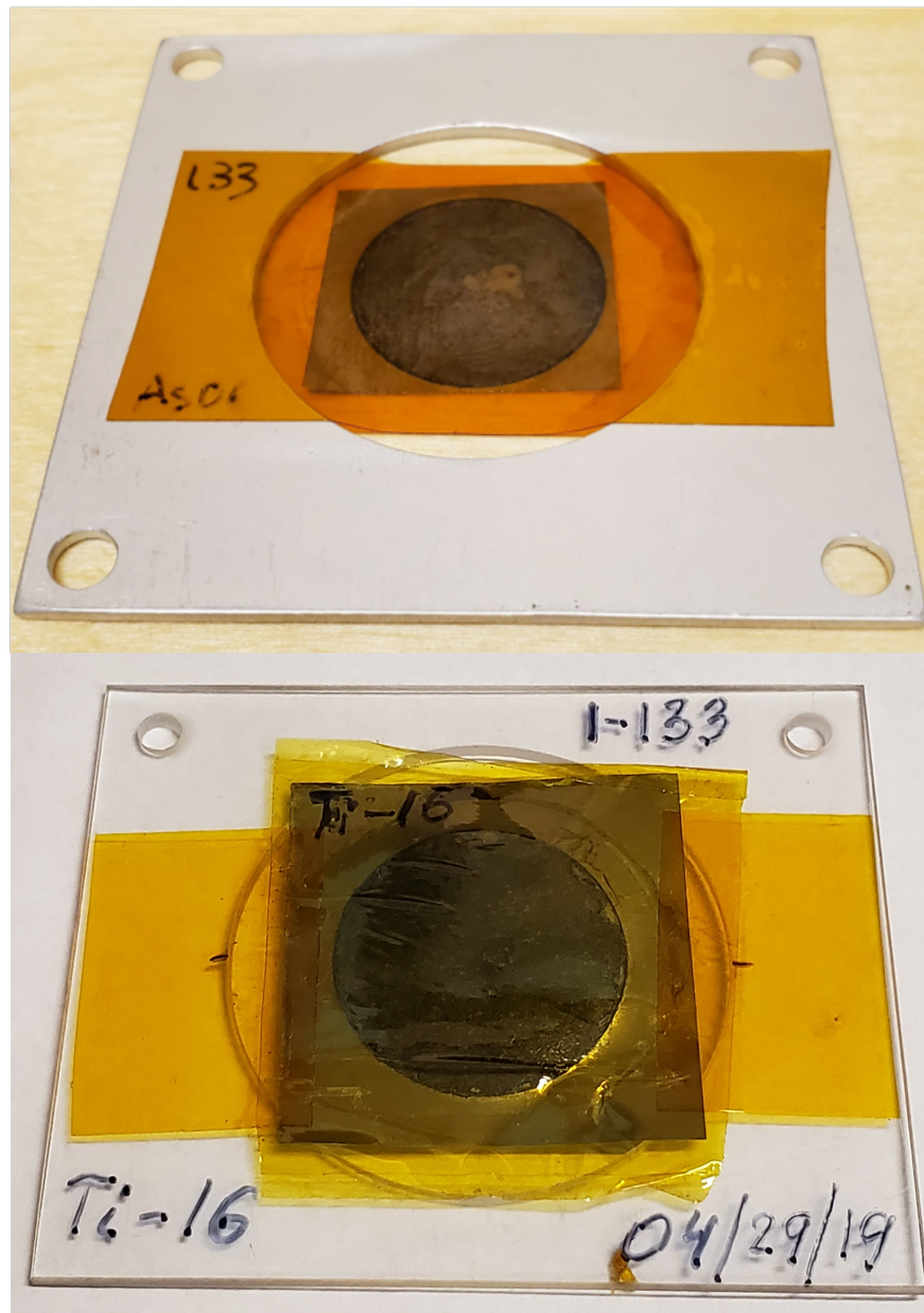
Figure 3.1: View of individual electroplated arsenic depositions on titanium backings within Kapton seals. The top target is sampled from the LBNL stack and is pictured after proton irradiation, where slight bubbling in the Kapton seal exists as a result of beam heating. The bottom target is part of the BNL stack prior to proton irradiation.
